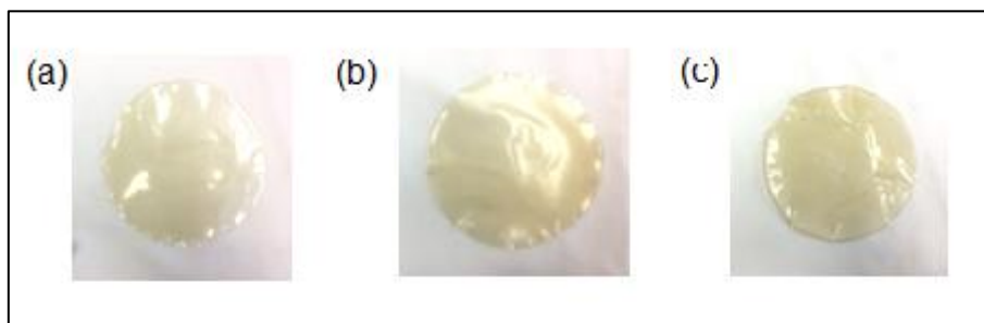
Figure 3.2. Appearance of biofilms from jackfruit seed starch; (a) 1% w/w starch-chitosan film, (b) 3% w/w starch-chitosan film, (c) 5% w/w starch-chitosan film
